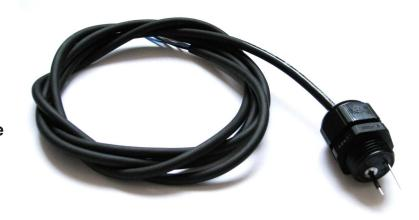
Liquid sensor type DRS-303 is designed for conducted liquid presence detection. Parameters of the detector have been fixed to allow detection of actual presence of liquid on its electrodes and to be resistant for low impedance conducted surfaces (eg. wet fingers). Additional reference electrode prevents detector against false signalling when liquid covers its surface only. PUSH-PULL output gives an opportunity for connection either to devices equipped with direct or inverse logic inputs.
