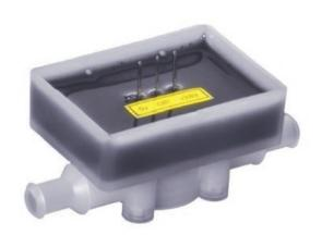
At the heart of the meter is a precision turbine that rotates freely on robust sapphire bearings and contains chemically resistant ceramic magnets that are detected through the chamber wall by a low power detector. The output is a stream of pulses that are readily interfaced with most electronic display or recording devices. This combination of materials and technology ensures a long life product with reliable operation throughout.
