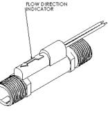
UNIT SPECIFICATION: - MOUNTABLE IN ANY ORIENTATION - TEMPERATURE RANGE UP TO 85 °C - PRESSURE TO 10 BAR (20 °C)
