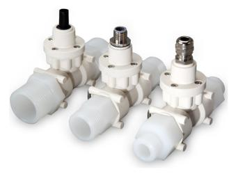
This multi-range radial flow turbine meter uses a low inertia turbine supported on robust sapphire bearings in a chemically resistant housing. Nine flow ranges (0.05 to 160 L/min), a choice of "plug in" fittings and individual traceable calibration make this meter one of the most flexible available.
