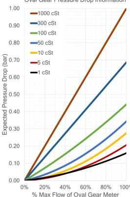
The rugged OG7 oval gear flowmeter is designed to give high performance with a low cost of ownership. It has a standard flow range from 5.0 to 500 L/min on 30 cSt oil and 20 to 500 L/min on water-like liquids. The standard inlet and outlet are 2" female threads. For OEMs, alternatives are available, including manifold mountings. The standard model is 316 St St with Viton™ 'O' ring seals.
