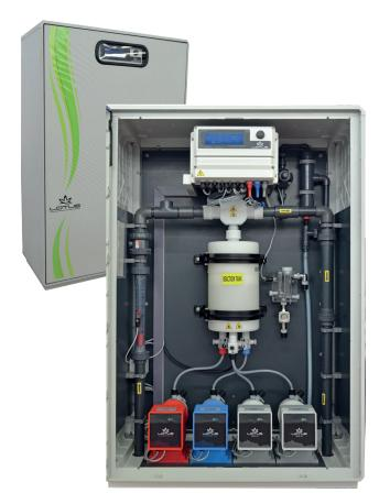
The chlorine dioxide generator named "LOTUS ULTRA" is used to produce liquid chlorine dioxide. This disinfectant kills all bacteria, germs, viruses and fungi very rapidly and works at very low concentration. The generator works according to the hydrochloric acid - chlorite process and uses diluted chemicals such as hydrochloric acid (HCI) and sodium chlorite (NaClO<sub>2</sub>) in accordance with the following chemical formula:
