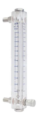
The LB/89 series flowmeters are designed for laboratory use suitable for small flow rates of liquid or gaseous fluids. Body in Plexiglas.
