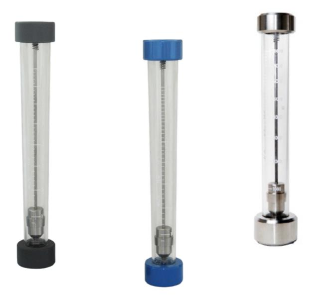
The "V-VK" series flowmeters are flow rate measuring devices, suitable for medium and large flow rates of liquid and gaseous fluids. The instantaneous measurement of the flow is read with excellent accuracy on the graduated scale, printed on the calibrated truncated-conical pipe in polycarbonate (makrolon) or polysulphone (non-toxic and unbreakable).
