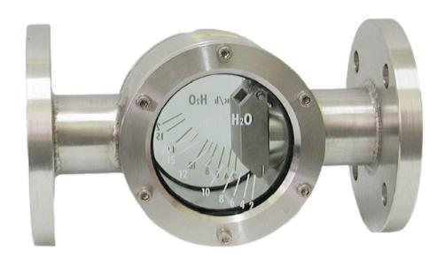
These are flow indicators for the visual control of liquids in industrial process and for the external mechanical detection of very dirty liquids. They are produced in different materials, with freeflow mobile blade pointer. The connections can be axial, either threaded or flanged. Maximum working pressure: 10 bars. The can be produced, on request, for PN16, PN25, Pn40. They can be only be mounted on horizontal pipe. Accurancy: ±10%.
