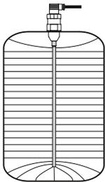
In the tank with straight wall (for example vertical cylinder) and with the sensor placed parallelly with the wall capacity change is linear.
