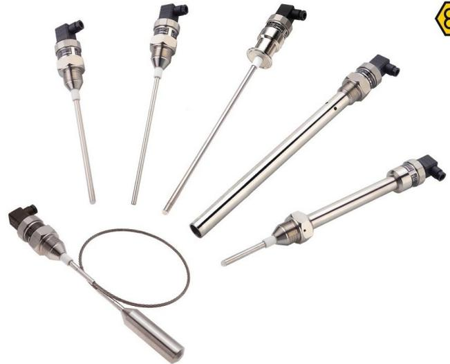
Capacitive level meters CLM® are designed for continuous level measurement of liquids, powders and bulk-solid materials in vessels, tanks, sumps, containers, silos, etc. CLM consists of the stainless steel housing with electronic module and the measuring electrode. The electronic part converts the capacity into the current signal (4 ... 20 mA) or voltage signal (0 ... 10 V). Sensitivity (SPAN) and initial capacity compensation (ZERO) can be fluently set.
