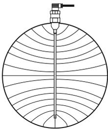
In a curved tanks (most frequently horizontal cylinder) capacity change during measuring of electrically non-conductive material is non-linear.
