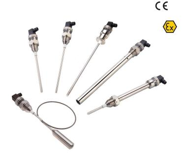
Capacitive level meters CLM® are designed for continuous level measurement of liquids, powders and bulk-solid materials in vessels, tanks, sumps, containers, silos, etc. CLM consists of the stainless steel housing with electronic module and the measuring electrode. The electronic part converts the capacity into the current signal (4 ... 20 mA) or voltage signal (0 ... 10 V). Sensitivity (SPAN) and initial capacity compensation (ZERO) can be fluently set.
