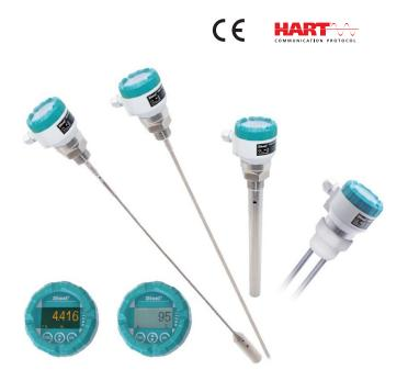
**Capacitive level meters CLM-70** are compact measuring devices consisting of the level meter body and a measuring electrode. The level meter body contains measurement electronics and a display module. The electronics measure the electrical capacity of the electrode system, which depends on the level height. The level meter's electrical output corresponds to the capacity (level height) and the measured data are shown on the meter's display.
