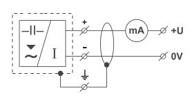
Fig. 2: Connection diagram of level meter with current output CLM-70\_-\_-I
