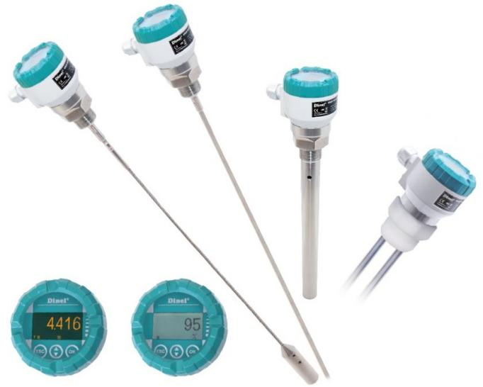
**Capacitive level meters CLM-70** are compact measuring devices consisting of the level meter body and a measuring electrode. The level meter body contains measurement electronics and a display module. The electronics measure the electrical capacity of the electrode system, which depends on the level height. The level meter's electrical output corresponds to the capacity (level height) and the measured data are shown on the meter's display.
