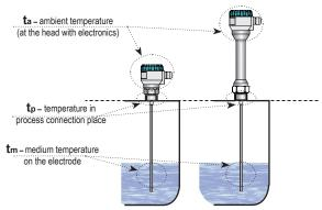
Fig. 1: Illustration of temperature measurement areas
