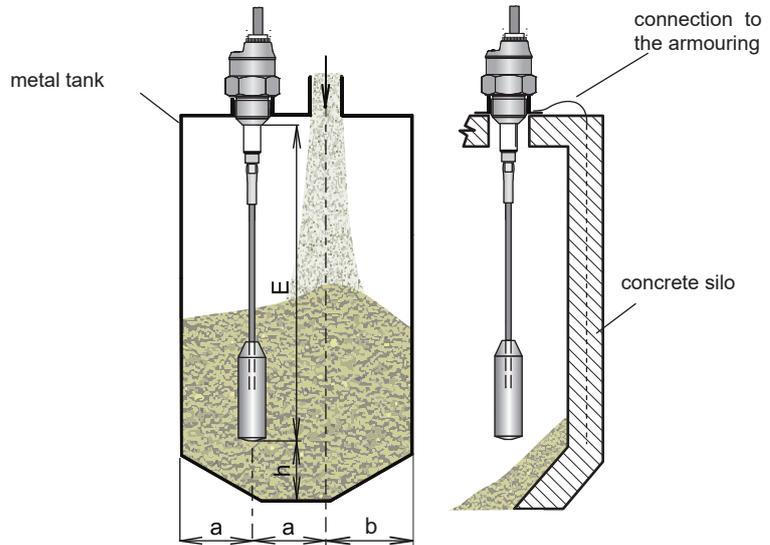
Installation of level meter with rope electrode
