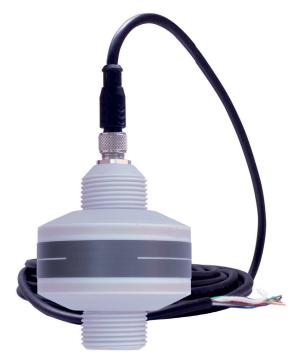
Range 0.05 ÷ 1.5 meters Blind zone 5 cm IP67|68 Suitable for measuring of liquids MODBUS RTU/BLUETOOTH comm. protocol Power supply 24 Vdc Output: 4 ÷ 20 mA analogue output
