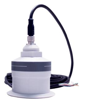
Range 0.3 ÷ 6 meters Blind zone 30 cm IP67|68 Suitable for measuring of liquids MODBUS RTU/BLUETOOTH comm. protocol Power supply 24 Vdc Output: 4 ÷ 20 mA analogue output Remote control via Smartphone
