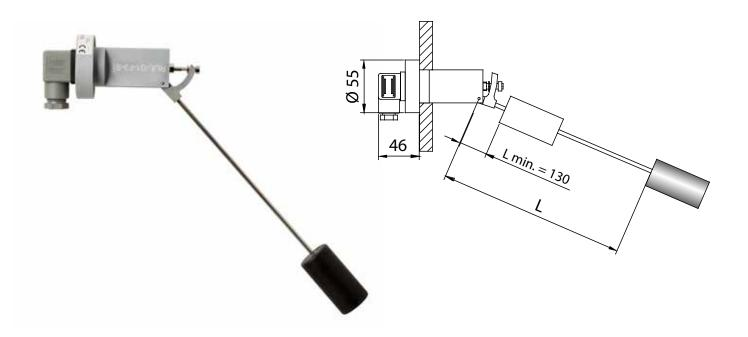
\* This level switch for "side" use is very versatile: like the "RL" range, it can also be used to control the maximum or minimum level and for controlling the minimum plus empty or maximum or overflow.
