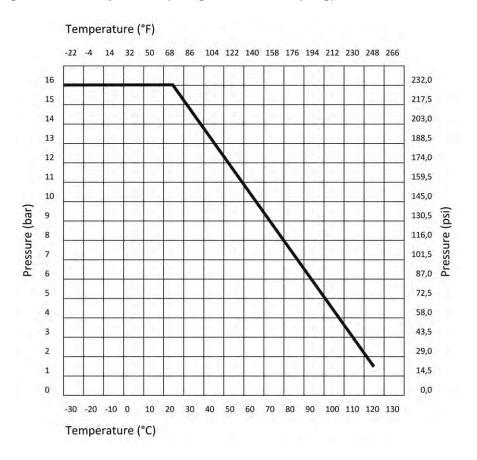
Data refers to water and non-hazardous fluids for which the material is classified as chemically resistant (25 years lifetime).
